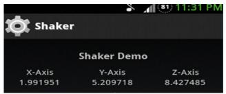
In this project a threshold value of 2 and -2 are being chosen but it can be generalised as per the needs of the user by virtue of which a user has to tilt his smart phone to certain desired angle and then press submit. In this way a user can set the various inputs as the various angles over which he wants to press a particular key from the keyboard.
